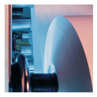
In the winding technology group you will find pneumatic tension brakes in various performance classes as well as elements for web tension control. With the tension brakes shown here, both relatively simple controls (with the use of Tensionor) and very complex web tension controls are possible.
