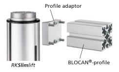
■ The profile adaptor allows several lifting columns to be together to form a stable combination. In this way, and with minimum effort, four columns can be connected to form lifting tables and operated via a synchronous control (MultiControl quadro). The aluminium profiles F-60/1, F-60-L, F-G 60, F-2G 60 from the BLOCAN® Profile Assembly System are suitable as struts for this purpose.
