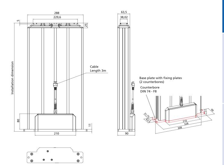
The fixing slots on the side allow an easy attachment of accessories. For example, a screen, CPU bracket or system reinforcements can be fixed to the lifting columns by using slot stones. The 30 slot geometry is also compatible with the RK BLOCAN® aluminium profile system.
