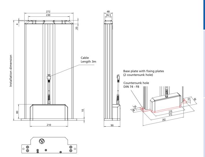
The fixing slots on the side allow an easy attachment of accessories. For example, a screen, CPU bracket or system reinforcements can be fixed to the lifting columns by using slot stones. The 30 slot geometry is also compatible with the RK BLOCAN® aluminium profile system.
