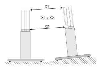
If the lifting columns are not parallel, the distance between the two upper fixing points will change during the movement. However, a rigid connection keeps this distance constant, and this means that the lifting columns are subject to very strong forces.
