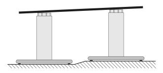
A rigid connection between the lifting columns aligns them at the same height. Fixing the table frame in place may cause the lifting columns to distort.
