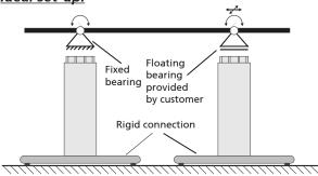
Surfaces at the foot and top of the columns must be at the same height, parallel to one another and as flat and even as possible, the columns themselves must also be aligned so that they are completely parallel. Existing tolerances and height differences due to control deviations are offset by means of a customer-provided floating bearing.
