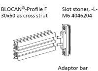
Code No. Version Adaptor bar for BLOCAN® profiles 4285000 Profile\* F-40 x 80-L, can be cut to specification Length (clear width between the Multilifts -2 mm)
