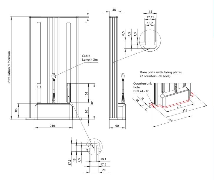
The fixing slots on the side allow an easy attachment of accessories. For example, a screen, CPU bracket or system reinforcements can be fixed to the lifting columns by using slot stones. The 30 slot geometry is also compatible with the RK BLOCAN® aluminium profile system.
